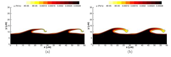
**FIG. 11.** Viscosity plots in the liquid phase for the three-dimensional planar jet at 150 bar with initial spanwise perturbation amplitude of 0.1  $\mu$ m. Different spanwise locations are shown at  $t = 3 \mu$ s. At this high pressure, the viscosity of the gas mixture remains within the range of 2.8–3.4 × 10<sup>-5</sup> Pa s. The interface location is highlighted with a solid black curve representing the isocontour with C = 0.5. (a)  $z = 5 \mu$ m; and (b)  $z = 15 \mu$ m.
