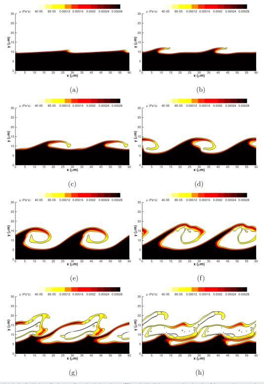
**FIG. 6.** Viscosity plots in the liquid phase for the two-dimensional planar jet at 150 bar. At this high pressure, the viscosity of the gas mixture remains within the range of 2.8–3.4 × 10<sup>-5</sup> Pa s. The interface location is highlighted with a solid black curve representing the isocontour with C = 0.5. (a)  $t = 1 \ \mu$ s; (b)  $t = 2 \ \mu$ s; (c)  $t = 3 \ \mu$ s; (d)  $t = 4 \ \mu$ s; (e)  $t = 5 \ \mu$ s; (f)  $t = 6 \ \mu$ s; (g)  $t = 7 \ \mu$ s; and (h)  $t = 8 \ \mu$ s.
