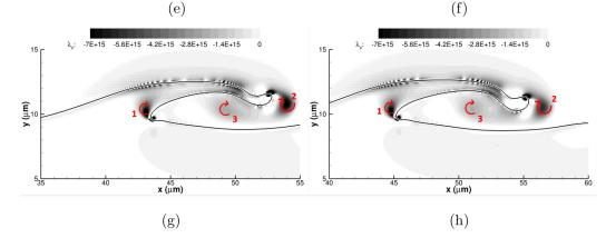
FIG. 17.  $\lambda_{\rho}$  contours for the two-dimensional planar jet at 150 bar. The red arrows point the rotation direction of the vortex. The interface location is highlighted with a solid black curve representing the isocontour with C = 0.5. (a)  $t = 1 \ \mu$ s; (b)  $t = 1.3 \ \mu$ s; (c)  $t = 1.6 \ \mu$ s; (d)  $t = 1.8 \ \mu$ s; (e)  $t = 2 \ \mu$ s; (f)  $t = 2.2 \ \mu$ s; (g)  $t = 2.5 \ \mu$ s; and (h)  $t = 2.7 \ \mu s.$
