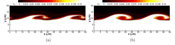
**FIG. 13.** *n*-decane mass fraction,  $Y_F$  plots in the gas phase for the three-dimensional planar jet at 150 bar with initial spanwise perturbation amplitude of 0.1  $\mu$ m. Different spanwise locations are shown at  $t = 3 \mu$ s. The interface location is highlighted with a solid black curve representing the isocontour with C = 0.5. (a)  $z = 5 \mu$ m; and (b)  $z = 15 \mu$ m.
