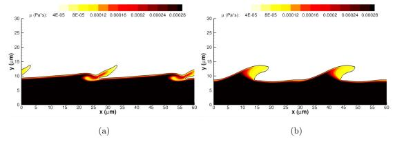
**FIG. 10.** Viscosity plots in the liquid phase for the three-dimensional planar jet at 150 bar with initial spanwise perturbation amplitude of  $0.5 \,\mu$ m. Different spanwise locations are shown at  $t = 3 \,\mu$ s. At this high pressure, the viscosity of the gas mixture remains within the range of  $2.8-3.4 \times 10^{-5}$  Pa s. The interface location is highlighted with a solid black curve representing the isocontour with C = 0.5. (a)  $z = 5 \,\mu$ m; and (b)  $z = 15 \,\mu$ m.
