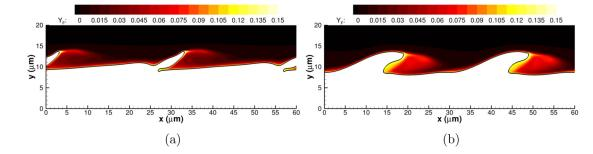
FIG. 12. *n*-decane mass fraction,  $Y_{5}$  plots in the gas phase for the three-dimensional planar jet at 150 bar with initial spanwise perturbation amplitude of 0.5  $\mu$ m. Different spanwise locations are shown at t=3  $\mu$ s. The interface location is highlighted with a solid black curve representing the isocontour with C=0.5. (a) z=5  $\mu$ m; and (b) z=15  $\mu$ m.
