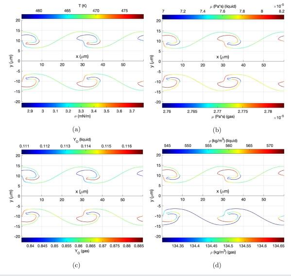
**FIG. 7.** Variation of various interface properties along the interface for the two-dimensional planar jet at 150 bar and  $t = 4 \ \mu$ s. The symmetry condition is used to mirror the jet and plot different variables on each side. The interface shape is colored by the value of each respective variable. (a) temperature, *T*, and surface tension coefficient,  $\sigma$ ; (b) viscosity,  $\mu$ ; (c) oxygen mass fraction, Y<sub>O</sub>; and (d) density,  $\rho$ .
