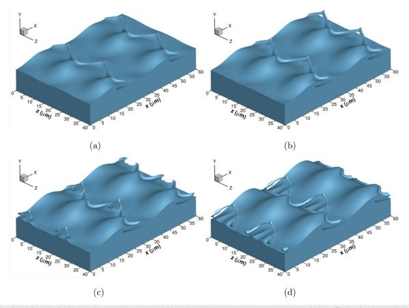
**FIG. 15.** Interface deformation for the three-dimensional planar jet at 150 bar with an initial spanwise perturbation amplitude of 0.3  $\mu$ m. The interface location is identified as the iso-surface with C = 0.5. (a) t = 2.5  $\mu$ s; (b) t = 2.8  $\mu$ s; (c) t = 3  $\mu$ s; and (d) t = 3.3  $\mu$ s.
