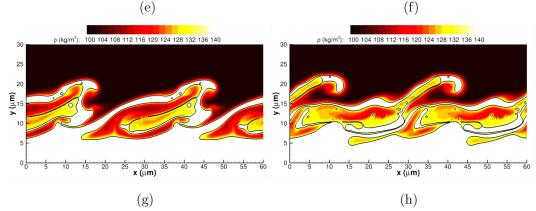
FIG. 4. Density plots in the gas phase for the two-dimensional planar jet at 150 bar. The interface location is highlighted with a solid black curve representing the isocontour with C = 0.5. (a)  $t = 1 \ \mu$ s; (b)  $t = 2 \ \mu$ s; (c)  $t = 3 \ \mu$ s; (d)  $t = 4 \ \mu$ s; (e)  $t = 5 \ \mu$ s; (f)  $t = 6 \ \mu$ s; (g)  $t = 7 \ \mu$ s; and (h)  $t = 8 \ \mu$ s.
