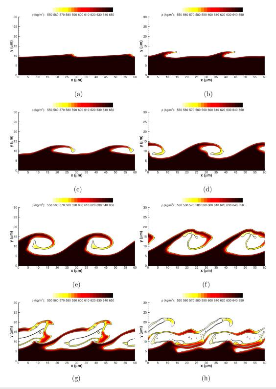
**FIG. 5.** Density plots in the liquid phase for the two-dimensional planar jet at 150 bar. The interface location is highlighted with a solid black curve representing the isocontour with C = 0.5. (a)  $t = 1 \ \mu$ s; (b)  $t = 2 \ \mu$ s; (c)  $t = 3 \ \mu$ s; (d)  $t = 4 \ \mu$ s; (e)  $t = 5 \ \mu$ s; (f)  $t = 6 \ \mu$ s; (g)  $t = 7 \ \mu$ s; and (h)  $t = 8 \ \mu$ s.
