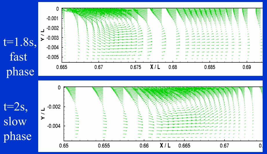
13°C, 1g, t=1.8s. Cold floor. Surface tension plus buoyancy causes recirculation.
