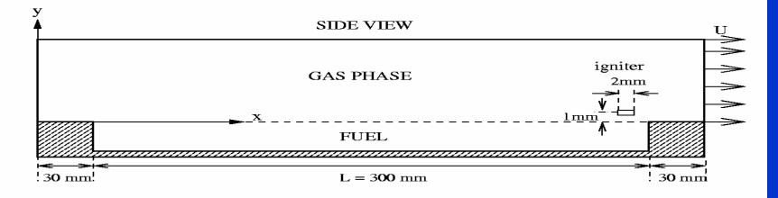
3-D Liquid Fuel Pool in wind tunnel floor. Igniter modelled as a hot gas pocket with a linear temperature increase to 1700 K in 0.01s.
