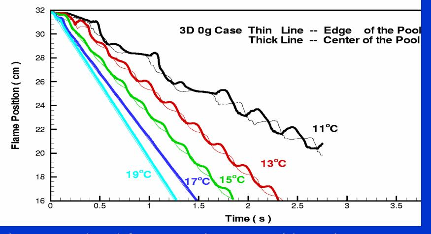
Flame speed and frequency increase with pool temperature.
