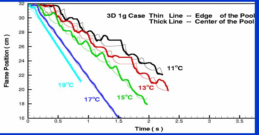
Flame speed and frequency increase with pool temperature. Pulsations occur at both 1-g and 0-g.
