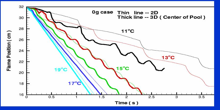
Flame speed and frequency increase with pool temperature.
