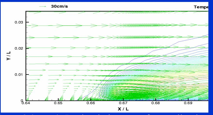
1g, t=2.0s, z=0. Recirculation zone forms allowing fuel vapor accumulation.
