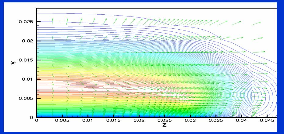
13 °C, 0-g, t=1.74s, x/L=.73. Cold floor. No vortex on side in absence of buoyancy.
