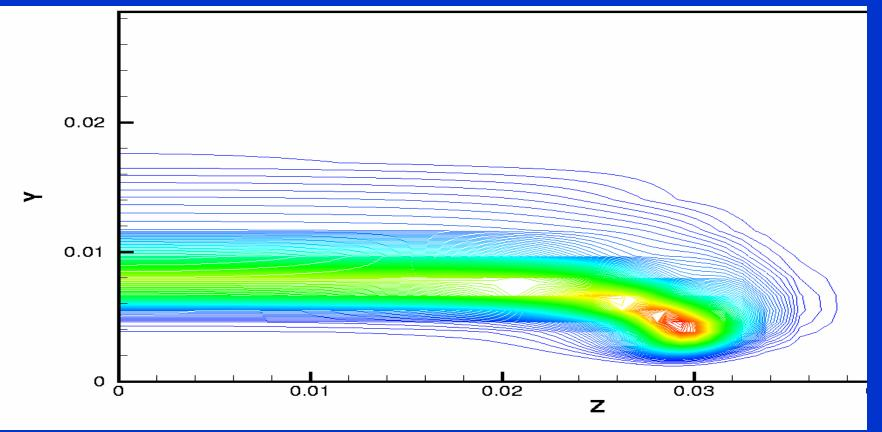
13 °C, pulsating case, 0-g, t=1.74s, x/L=.73. Cold Tunnel Floor.
