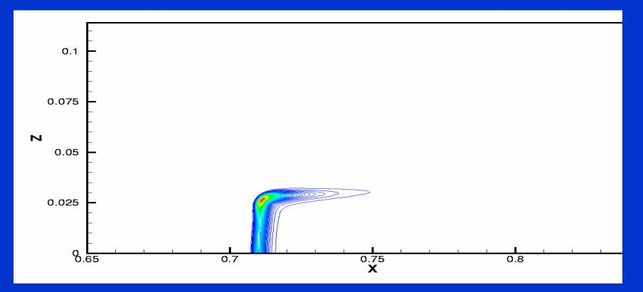
13 °C, pulsating case, 0-g, t=1.74s, y=1mm. Cold Tunnel Floor. Flame tails along pool edge are short.
