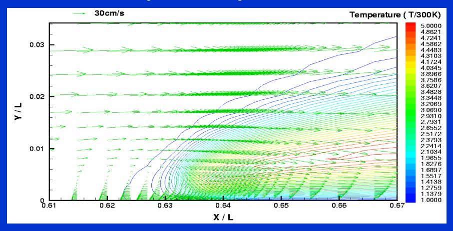
13°C, 0-g, t=2.3s, slow phase. Forced convection together with surface tension causes recirculation.
