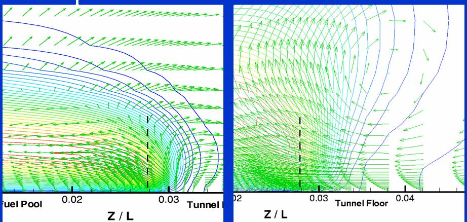
13°C, 1g, t=1.8s. Cold Floor. x/L=0.69; expansion near flame front. x/L=.75, recirculation.
