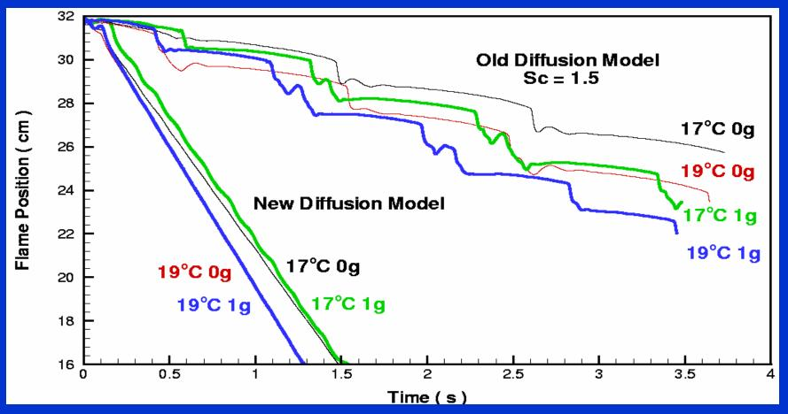
30 cm/s opposed flow. Flame speed and frequency increase with pool temperature. Pulsations occur at both 1-g and 0-g. Fast oxygen diffusion accounts for increased flame speed.
