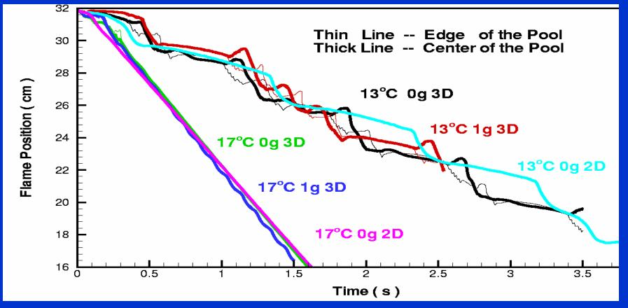
30 cm/s opposed flow. Flame speed and frequency increase with pool temperature. Pulsations occur at both 1-g and 0-g.
