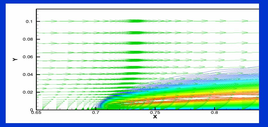
13°C, 0-g, t=1.74s. Flame remains close to surface in absence of buoyancy.
