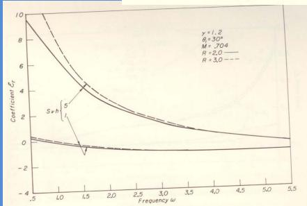
Fig. 16(a) Real part of combined admittance coefficient versus frequency: Effect of throat wall curvature
