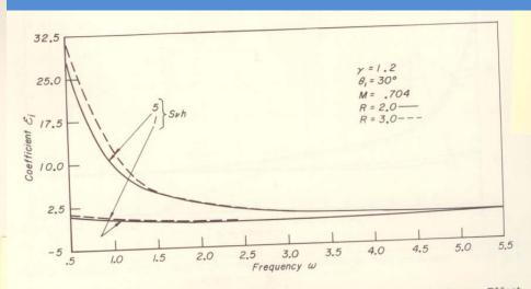
Fig. 16(b) Imaginary part of combined admittance coefficient versus frequency: Effect of throat wall curvature
