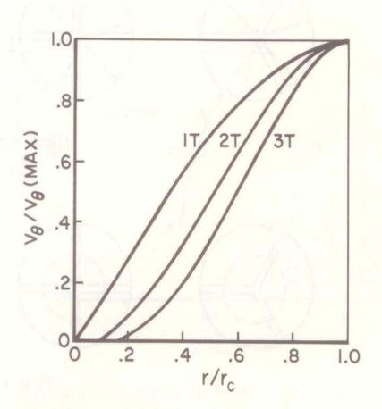
FIGURE 8.2.2c.—Tangential mode velocity profiles.
