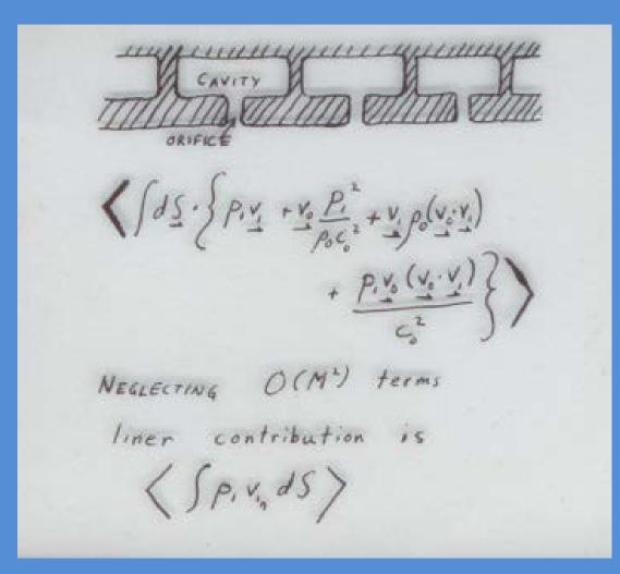
Acoustic Liners can be Helmholtz resonators, quarter wave tubes, or a hybrid of both.
