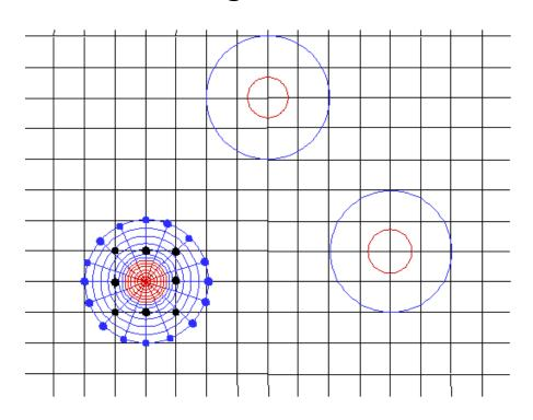
The computational domain is divided into N (number of droplets) liquid-phase spherical domains, N gas-phase spherical domains around the droplets, and one Cartesian domain outside of the gas-phase spherical domains.
