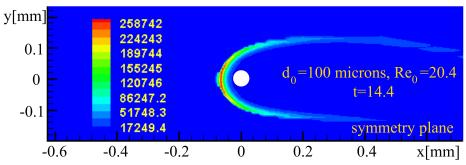
The flames (separated) for the case with initial diameter 100 microns, spacing 4.2  $d_0$ , and Re=20.4
