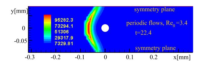
The flame (group) for the case with initial diameter 50 microns, spacing 4.2  $d_0$ , and Re=3.4
