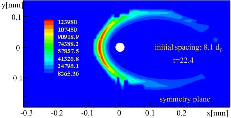
The flame (separated) for the case with initial diameter 50 microns, spacing 8.1 d<sub>0</sub>, and Re=3.4
