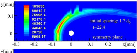
The flame (group) for the case with initial diameter 50 microns, spacing  $1.7d_0$ , and Re=3.4
