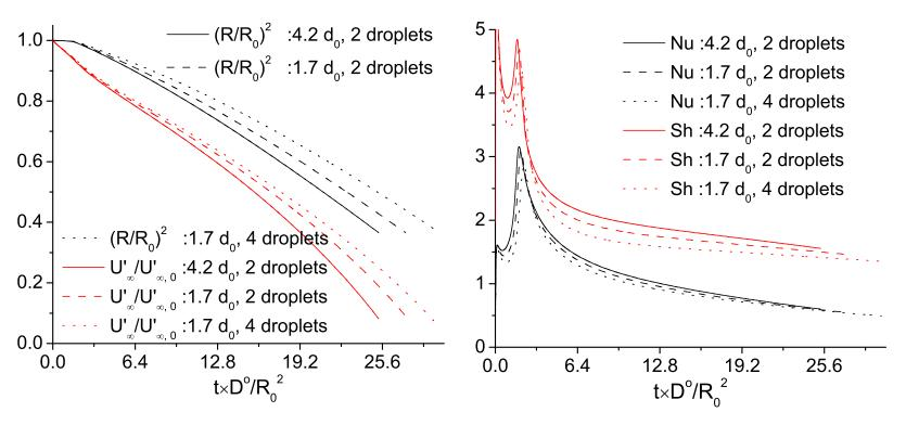
Comparisons of Radius squared, relative gas-droplet velocity, Nusselt number and Sherwood number for three cases with different array configurations and droplet spacing. The peaks in Nu and Sh are due to initial adjustment and ignition. ( $d_0$ =50microns, Re=3.4)
