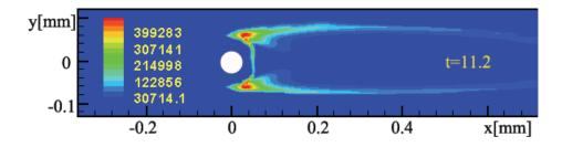
The flames (separated and wake) for the case with initial diameter 100 microns, spacing  $4.2~d_{_{0}}$ , and Re=81.6
