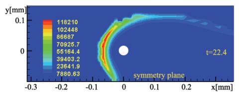
The flame (group) for the case with initial diameter 50 microns, spacing 4.2d<sub>0</sub>, and Re=3.4
