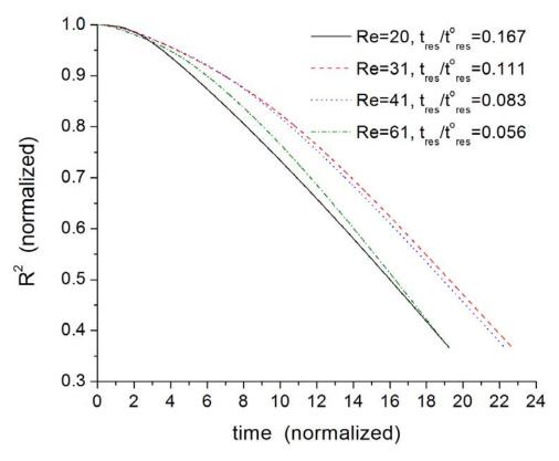
Comparisons of Radius squared for different initial relative velocity under the same initial diameter. As the initial relative velocity is increased, the initial residence time is decreased and the initial Reynolds number is increased, so this plot can be explained from the previous two plots.
