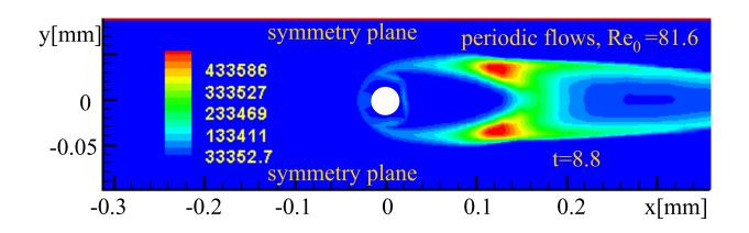
The flames (separated and wake) for the case with initial diameter 50 microns, spacing  $4.2~d_0$ , and Re=81.6
