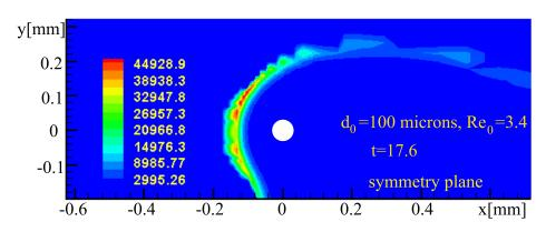
The flame (group) for the case with initial diameter 100 microns, spacing 4.2  $d_{\rm 0}$ , and Re=3.4
